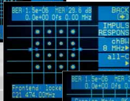
Constellation diagram of an OFDM signal (16QAM)
